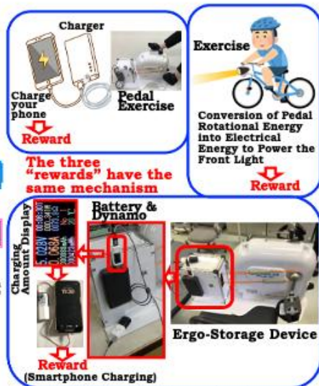
Fig. 1(b) The ergo-storage device developed in this study to promote exercise implementation and continuation.
